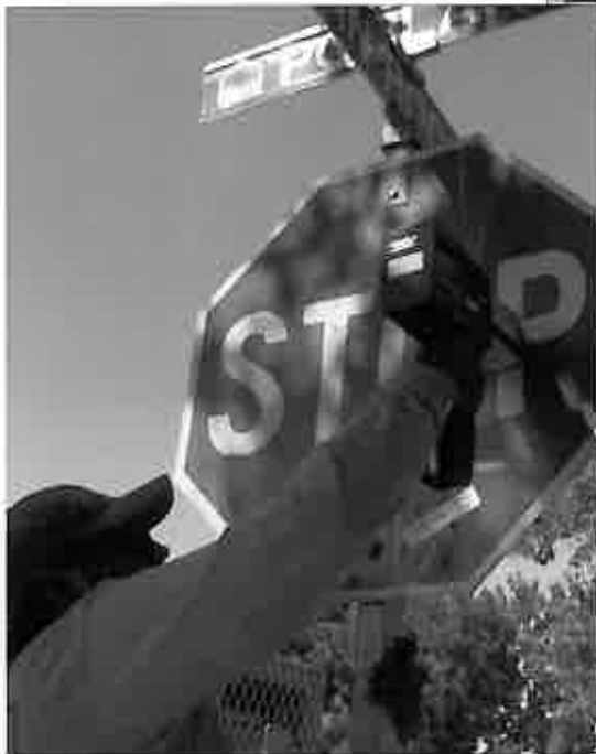
A RetroSign retroreflector gun enabled with GPS allows public works staff to collect sign location and sign reflectivity at once. That data is then managed in a GIS-enabled asset management system.
